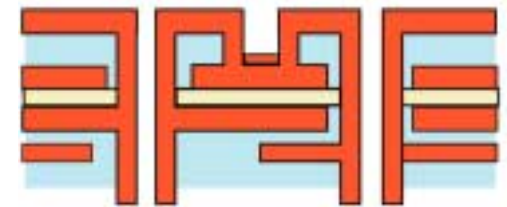
THROUGH HOLE AND MICRO VIA FORMATION
